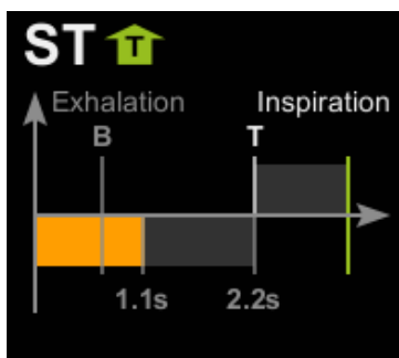
Variant D: Controlled ventilation with blocked trigger impulse
