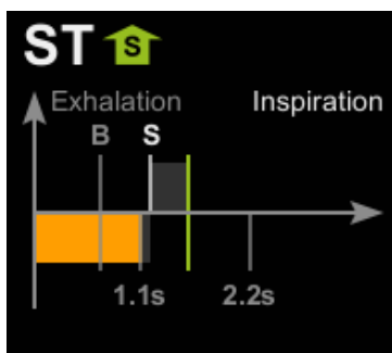
Variant B: Spontaneous breathing with blocked trigger impulse
